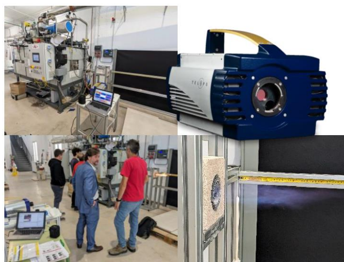
Figure 1. Combustion study system with controlled gas input in ITC'S facilities. The multi-spectral aligned in front the output flame.
