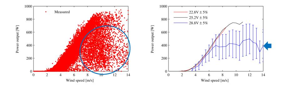
Following IEC standard, the systems includes the charge controller and the dump load. The charge controller is connected in parallel to the generator rectified output. It diverts the energy to the dump load when the battery voltage rises above a preset level (26.4 V here). This happens when the battery is fully charged or during wind gusts. The resulting effect can clearly be seen on the 28.8V  $\pm$  5% power curve: the output power has a large standard deviation and drops in average.
