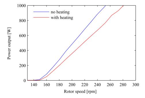
Small-scale axial flux generators can have important localized heating because of (1) their high power density, and (2) their poor thermal design in comparison with large-scale machines. To illustrate the potential impact of generator heating on electrical output power, we carried out test bench measurements. The scattering caused by generator heating can reach 50 W at 175 RPM. This gives us an upper bound on power loss due to machine heating.
