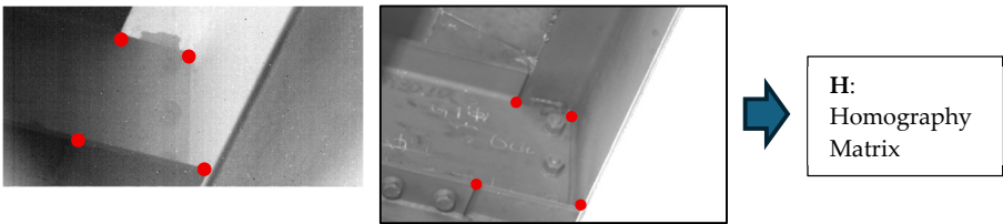
Figure 6. Calculate Homography Matrix(H)
