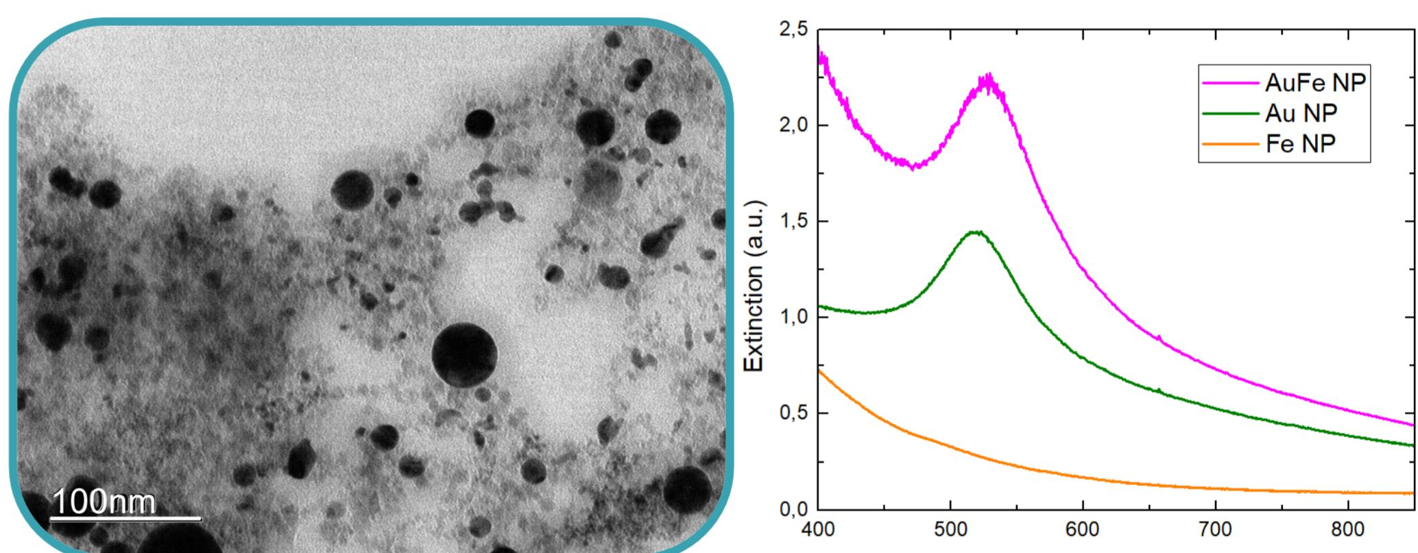
Left: TEM image corresponding to AuFe NP at 50,000x magnification. Right: UV-Vis measurements indicating the colloidal extinction spectra. Inset: DLS for colloidal AuFe NP.
