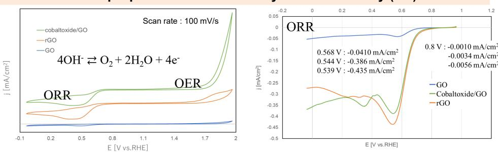
Electrochemical analysis showed pronounced ORR and OER catalytic activity of the synthesized CoO/GO composite materials
