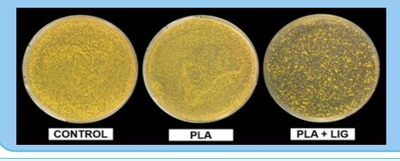
Left) Fewer *Micrococcus Luteus* colonies (yellow dots) were observed on the electrospun PLA+Lignin membrane compared to the control and PLA-only membranes, where colonies densely covered the surface.
