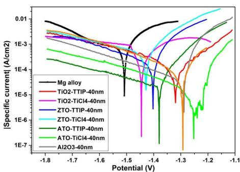
Results of the corrosion tests
