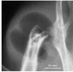
Biodegradation of magnesium-based screw
