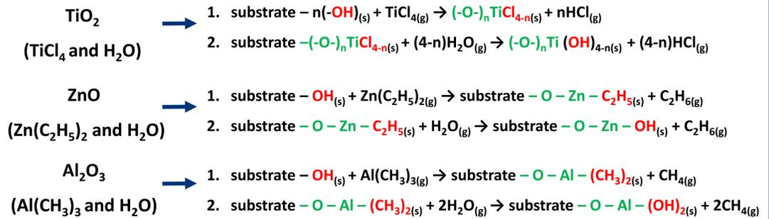
Scheme of Al<sub>2</sub>O<sub>3</sub> synthesis by ALD method
