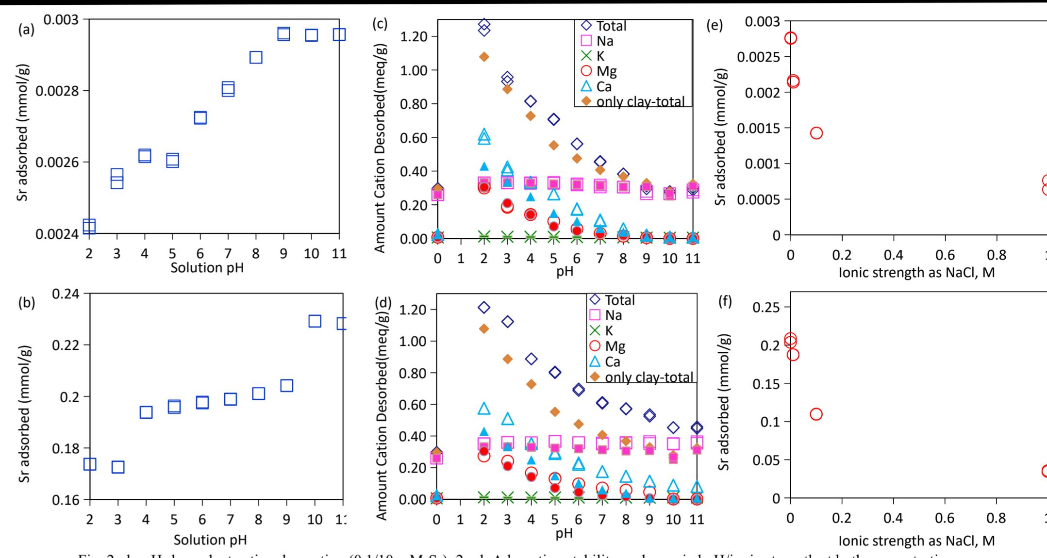
Fig. 2a-b: pH-dependent cation desorption (0.1/10 mM-Sr). 2c-d: Adsorption stability under varied pH/ionic strength at both concentrations. 2e-f: Ionic strength effects on Sr<sup>2+</sup> adsorption.
