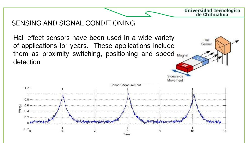
International Electronic Conference on Sensors and Applications 1 - 16 June 2014 In order to detect the speed of the motors' shaft, there are placed three permanent magnets equally spaced at 120°, whose magnetic fields can be detected by a fixed Hall effect sensor
