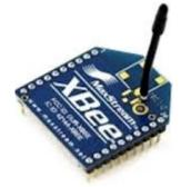
Wireless transmission and reception is done by two Xbee RF modules working in transparent mode, this implies that, all UART data received in the transmission module is queued for RF transmission. When RF data is received by the reception module, it is transmitted to the data analysis block to later be displayed
