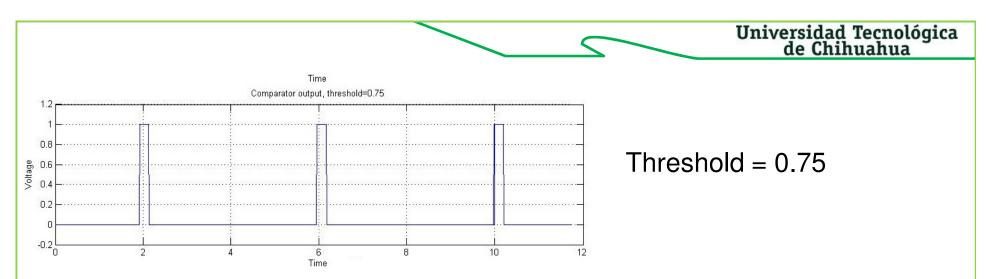
By changing the threshold parameter in the comparator, the pulse width is modified. Greater thresholds carry thinner pulses, while lower thresholds implies wider pulse trains.
