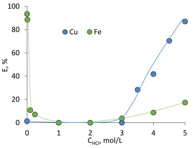
HES TIBPS/octanoic acid allows the separation of metal ions at both low and high concentrations of hydrochloric acid with high separation coefficients ( $\beta_{Cu/Fe}$ =31.97 at 5 M HCl and  $\beta_{Fe/Cu}$ =1061.92 at <1M HCl).
