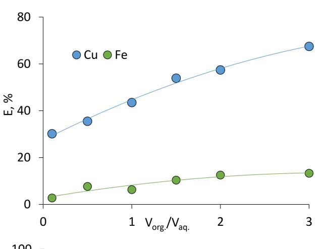
The separation of the Cu/Fe pair can be optimized by varying the volume ratio of the phases. The best results were obtained at an HCl concentration of 3.5 M with a phase ratio (Vorg./Vaq.) of 3.
