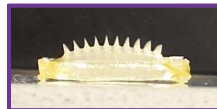
Figure 3. The obtained microneedle patch.
