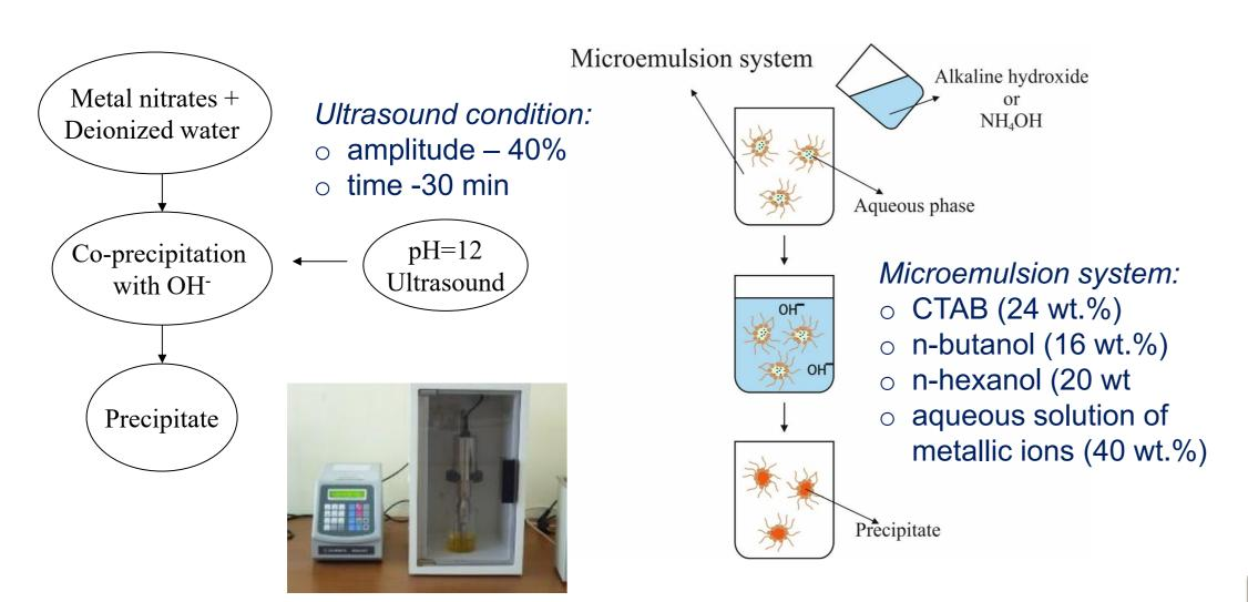
The molar ratio of Ba to Fe is 1:10. The co-precipitation process was caused by adding NaOH at pH12. The precursors are synthesized at  $800^{\circ}\text{C}$  and  $900^{\circ}\text{C}$  to obtain  $\text{BaFe}_{12}\text{O}_{19}$ .
