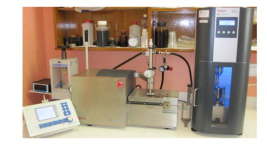
Laboratory equipment for wood-plastic composite processing **HAAKE MiniLab II and MiniJet II, (Thermo Scientific)**
