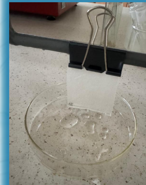
Fig. 6. Photograph of a sample during water drainage (water absorption tests).
