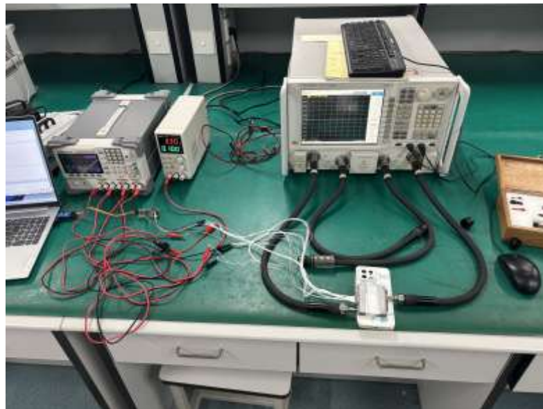
Figure 8. Physical picture of TR component vector network test.
