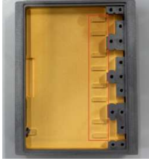
Figure 5. Physical picture of the box body and position of the amplifier chip stage.
