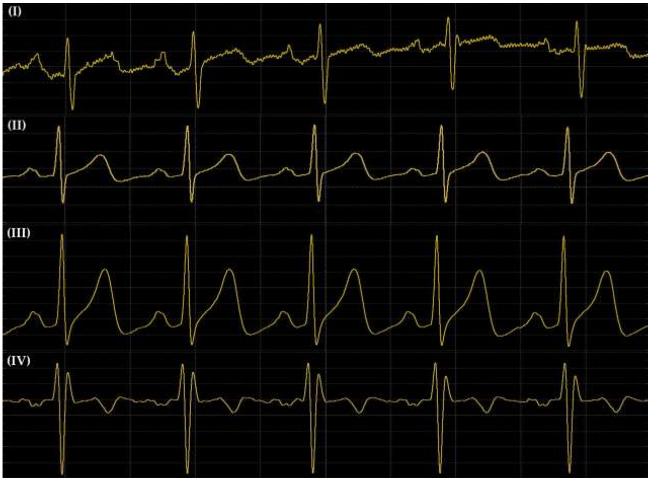
Figure 8. Signals acquired using (I) the commercial board based on the SparkFun design, (II) the AFE board design with the Cardiac monitor configuration application, (III) the AFE board design with the Portable cardiac monitor with elimination of motion artifacts application, and (IV) the AFE board design with the Exercise application: heart rate measured at the hands.
