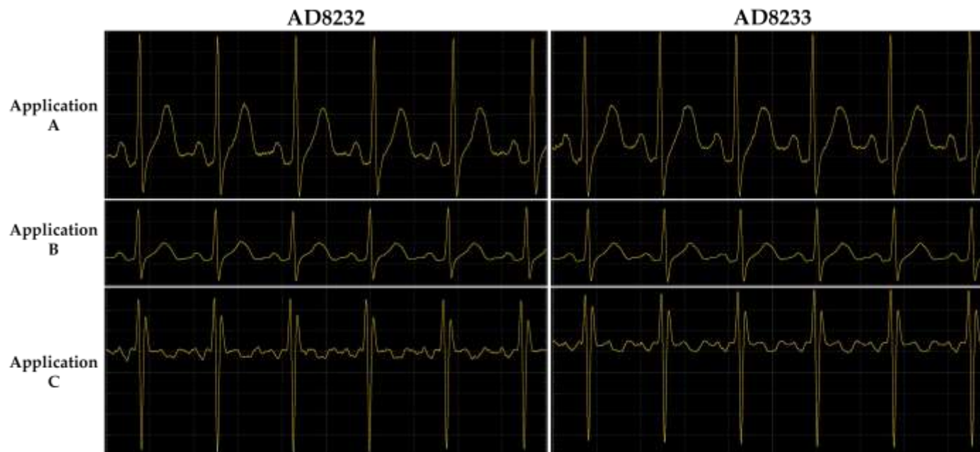
Figure 7. Signals acquired on the breadboard using the AD8232 and AD8233 chip adapters where application (A) Cardiac monitor configuration, application (B) Portable cardiac monitor with elimination of motion artifacts and (C) Exercise application: heart rate measured at the hands.
