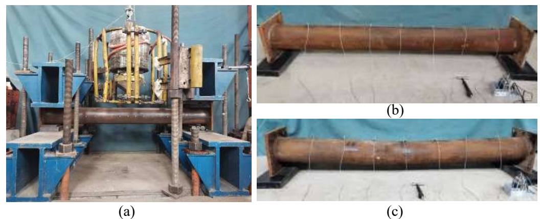
Figure 3. Experimental setup of lateral impact testing on CFST specimen. (a) Lateral impact testing apparatus (b) Intact CFST specimen before impact, and (c) Damaged CFST specimen after impact.
