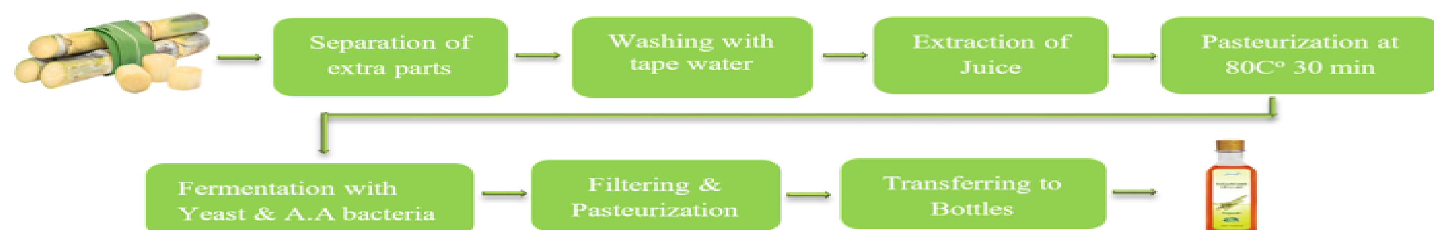
Figure 2. This diagram shows the schematic representation of sugarcane vinegar production process.
