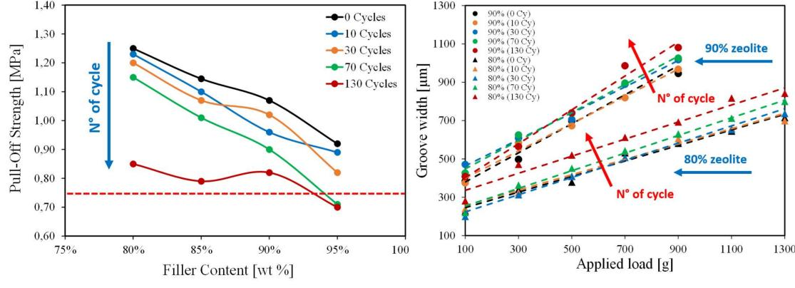
The coating's pull-off resistance remained stable initially but experienced a progressive decrease after 70 aging cycles, eventually stabilizing at 0.8 MPa. This reduction in adhesion is caused by vapor penetration at the interface. The 90% zeolite formulation proved to be the most mechanically stable, effectively balancing polymer permeability and matrix instability.
