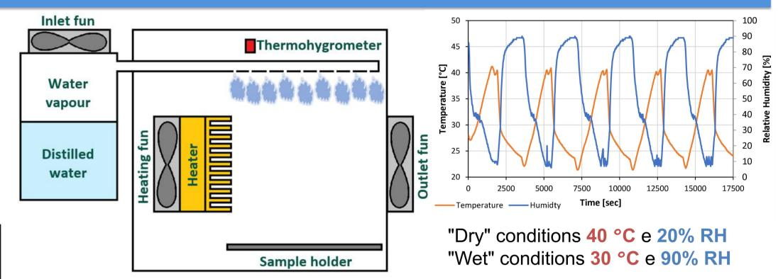
A prototype climatic chamber was developed to simulate wet/dry cycles. This chamber is thermally insulated and connected to a steam generator. Inside, a heating element coupled with a fan maintains the set temperature, while a second fan exhausts internal humidity to the outside.
