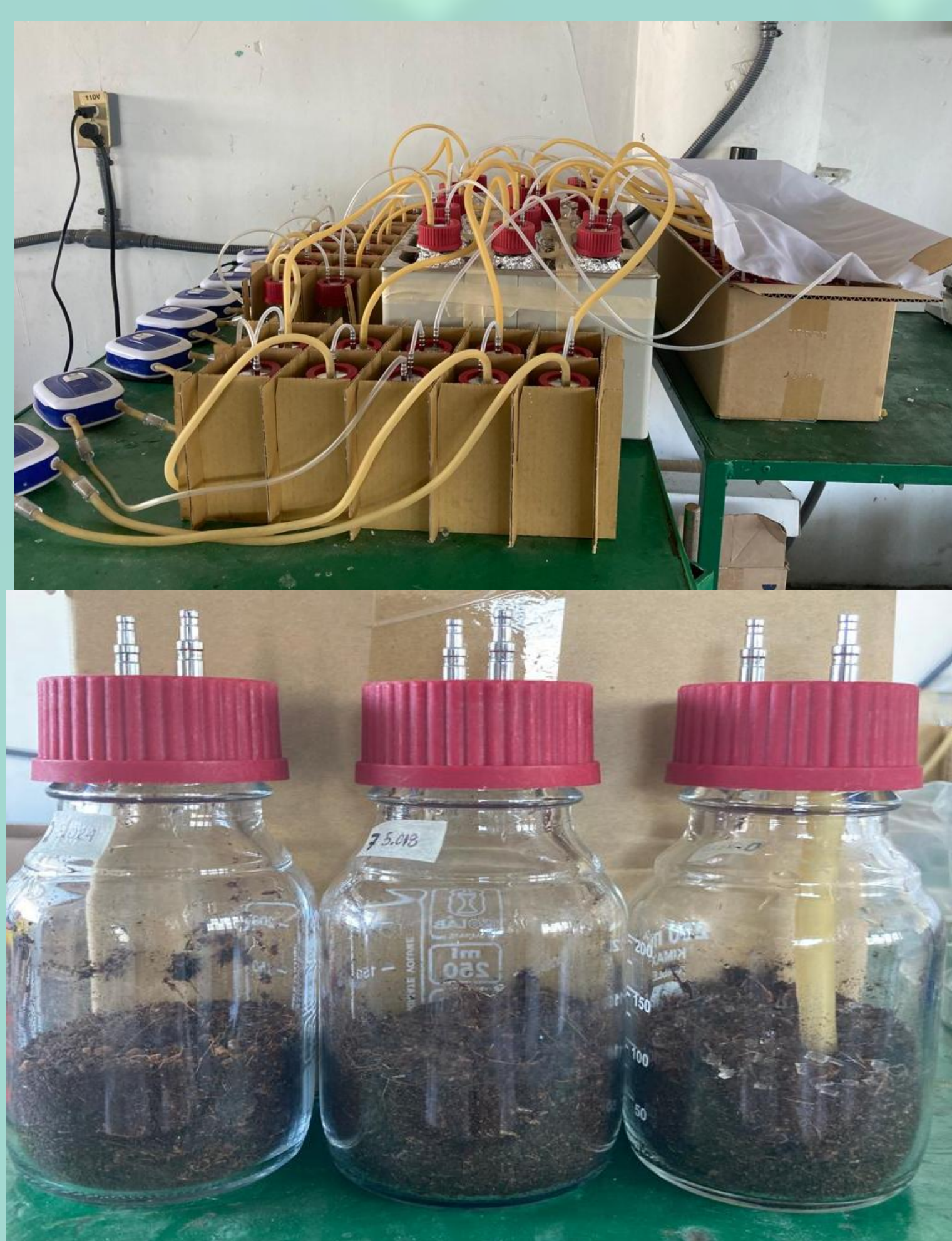
Figure 1. Biodegradation system for CO 2 evolution. (Top) System. (Bottom) Biological reactors
