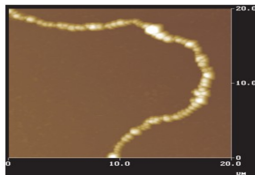
AFM scan of a magnetic filament. After K Erglis et al., J. Phys.: Condens. Matter 20 , 204107 (2008)
