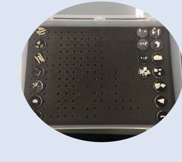
4. Specimen mounted on to stubs for SEM imaging.
