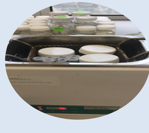
3. Sonic water bath (5 min) to remove excess organic matter
