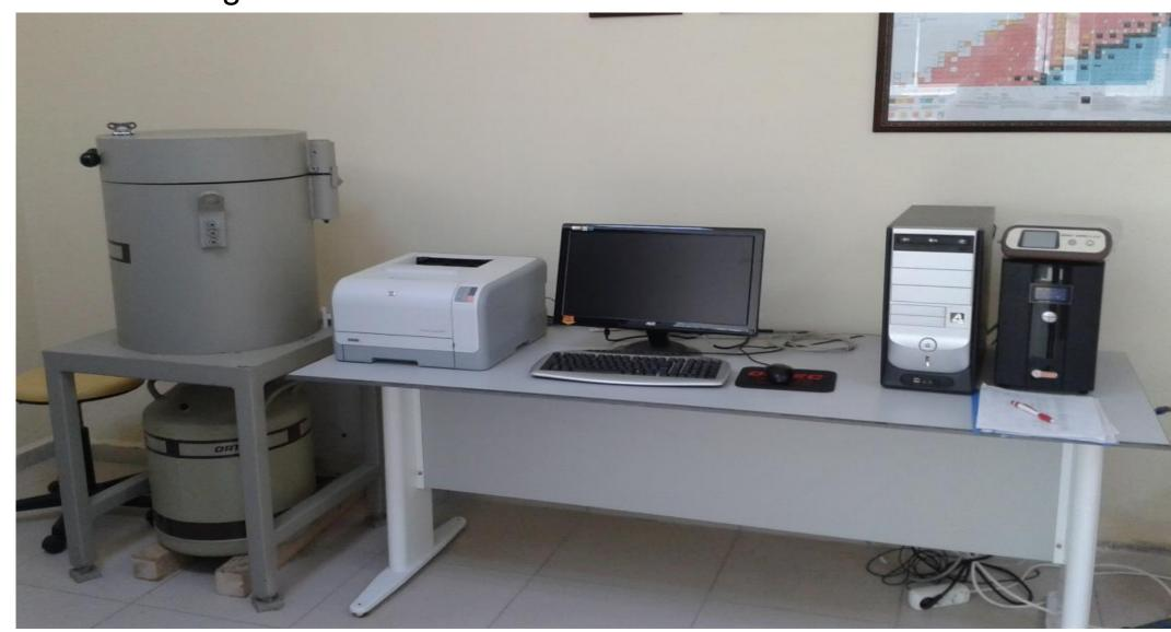
Each concrete sample was counted in the detector for 86,400 s (one day), and the resulting spectra were analysed using the Gamma Vision program. An empty plastic measuring cup, under the same measurement conditions as the samples, was also counted in the detector to determine background concentrations. These background contributions were subtracted when evaluating the sample spectra.
