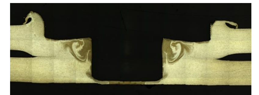
Figure 7. OM micrograph of a GNP-reinforced FSSW joint.
