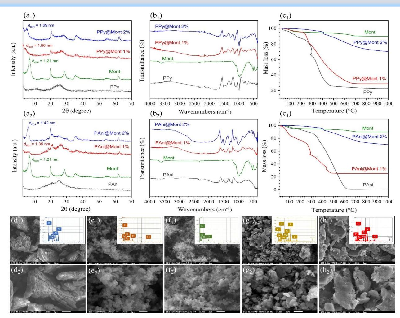
Structural, thermal, and morphological characterization of bare montmorillonite, PPy, PAni, and their polymer@montmorillonite composites: (a1, a2) XRD patterns, (b1, b2) FTIR spectra, (c1, c2) TGA curves, and SEM-EDX micrographs of (d1, d2) montmorillonite, (e1, e2) PPy, (f1, f2) PAni, (g1, g2) PPy@Mont, and (h1,h2) PAni@Mont.
