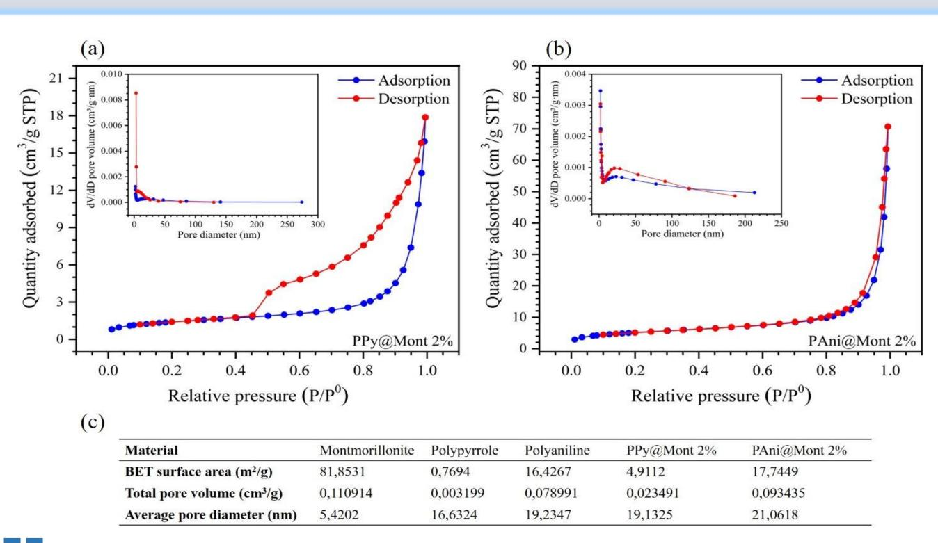
Nitrogen adsorption-desorption isotherms (77 K) and BJH pore-size distribution (inset) of PPy@Mont (a) and PAni@Mont (b). BET surface area, total pore volume, and average pore diameter of pristine Mont, PPy, PAni, and their composites (c).
