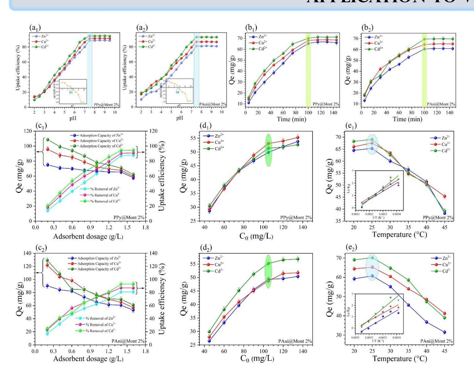
Adsorption behavior and thermodynamic analysis of Zn<sup>2+</sup>, Cu<sup>2+</sup>, and Cd<sup>2+</sup> on PPy@Mont and PAni@Mont composites: (a1, a2) Effect of pH on the percent removal (%) (Inset: plot showing the point of zero charges), and effect of (b1, b2) contact time, (c1, c2) adsorbent dosage, (d1, d2) preliminary heavy metal concentration, and (e1, e2) temperature on the adsorption capacity (Qe, mg/g) (inset: Van't Hoff plots).
