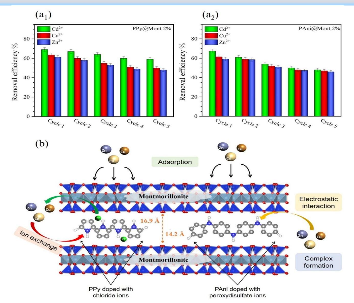
Reusability performance of PPy@Mont and PAni@Mont composites over five adsorption-desorption cycles for Cd<sup>2+</sup>, Cu<sup>2+</sup>, and Zn<sup>2+</sup> ions (a1, a2), and representation of suggested adsorption mechanisms involving electrostatic interaction, ion exchange, and metalligand complexation between metal ions and CP@Mont composites.
