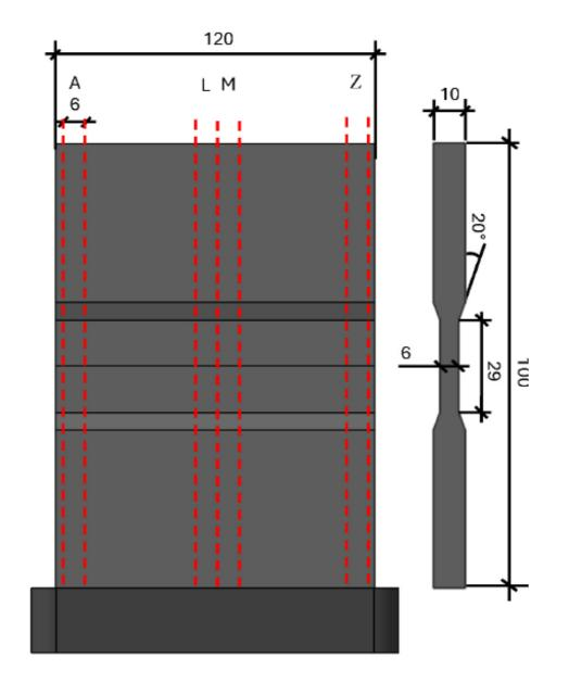
These different orientations have **distinct heat dissipation rates** and **thermal histories** for the material as it solidifies. **Vickers microhardness** tests are done and, also grain size analysis following the standard procedure set out in ASTM E112.
