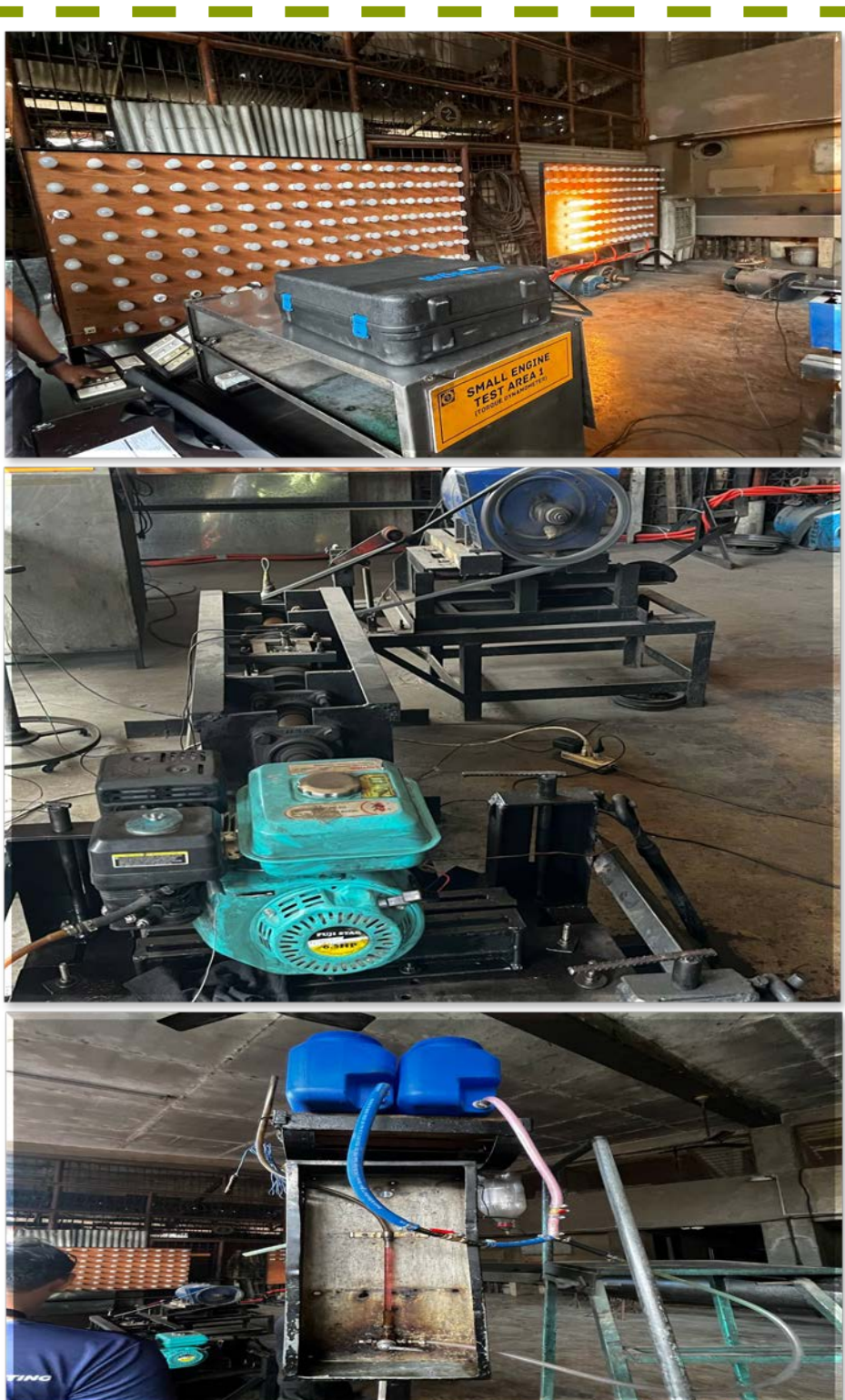
Varying Speed Test (Load Simulation Setup)
