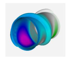
The inflow of liquid causes changes in the liquid film pressure. The greater the inflow rate, the greater the effect.
