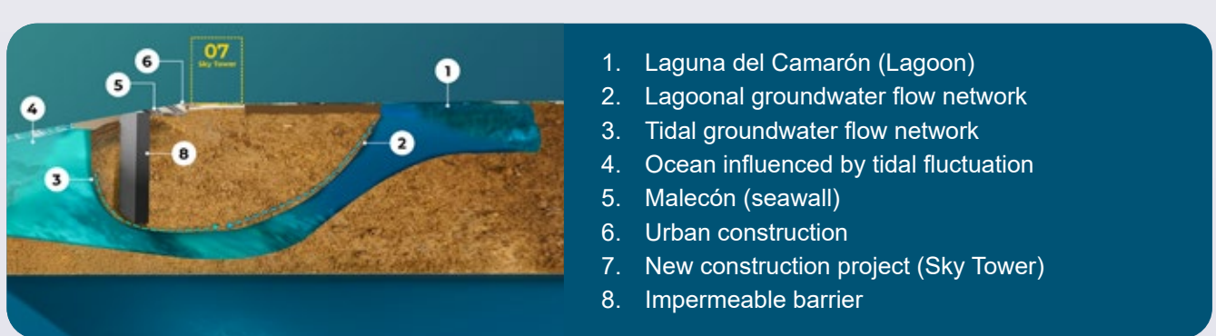
Figure 4. Representative Groundwater Flow Network
