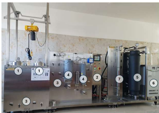
Figure 2. Front view of supercritical CO 2 extraction equipment: 1-feed tanks; 2-extraction control system, 3-valves, 4-extracted sample collection valves, 5-CO 2 tanks, 6-cold water tank, 7-CO 2 level meter.
