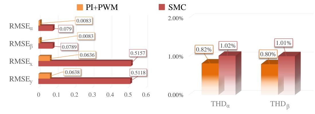
Fig. 5: SMC vs. PI+PWM controller performance: RMSE [A] and THD results at 12 kHz and 1000 r/min.
