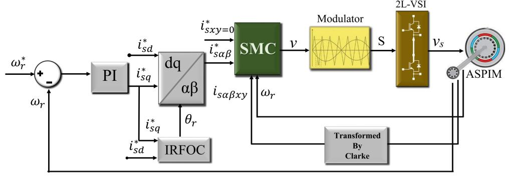
Fig. 3: Block diagram of the SMC system for the ASPIM.
