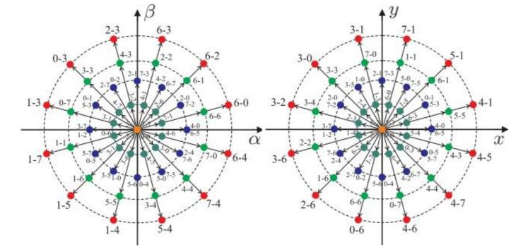
Fig. 1: Space voltage vector in the  $(\alpha - \beta)$  and (x - y) subspaces. [2]
