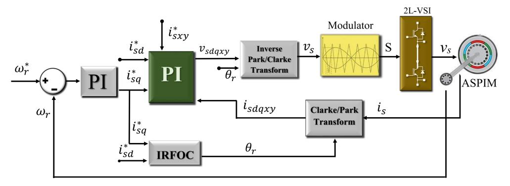
Fig. 2: Block diagram of the PI+PWM system for the ASPIM.
