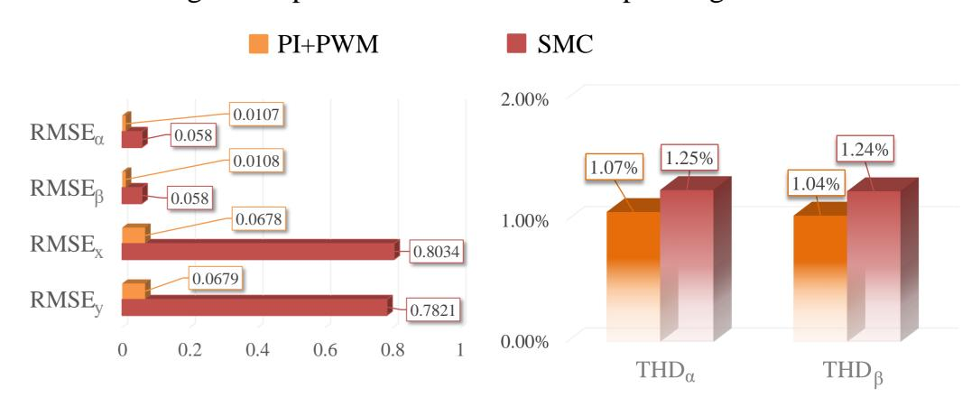
Fig. 4: SMC vs. PI+PWM controller performance: RMSE [A] and THD results at 8 kHz and 500 r/min.
