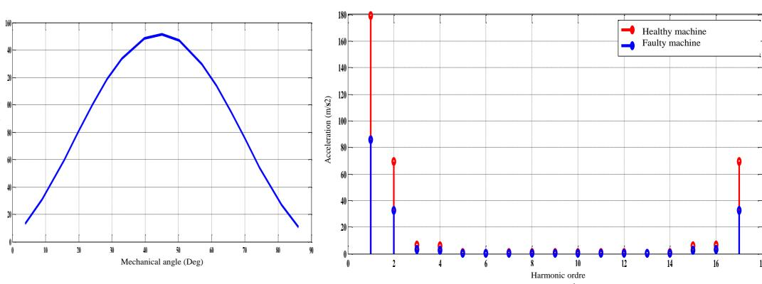
Bar breakage causes a reduction in the mean electromagnetic torque while simultaneously increasing the amplitude of its oscillations. This, in turn, enhances the magnetic forces and consequently increases the oscillations of the rotational speed (acceleration).
