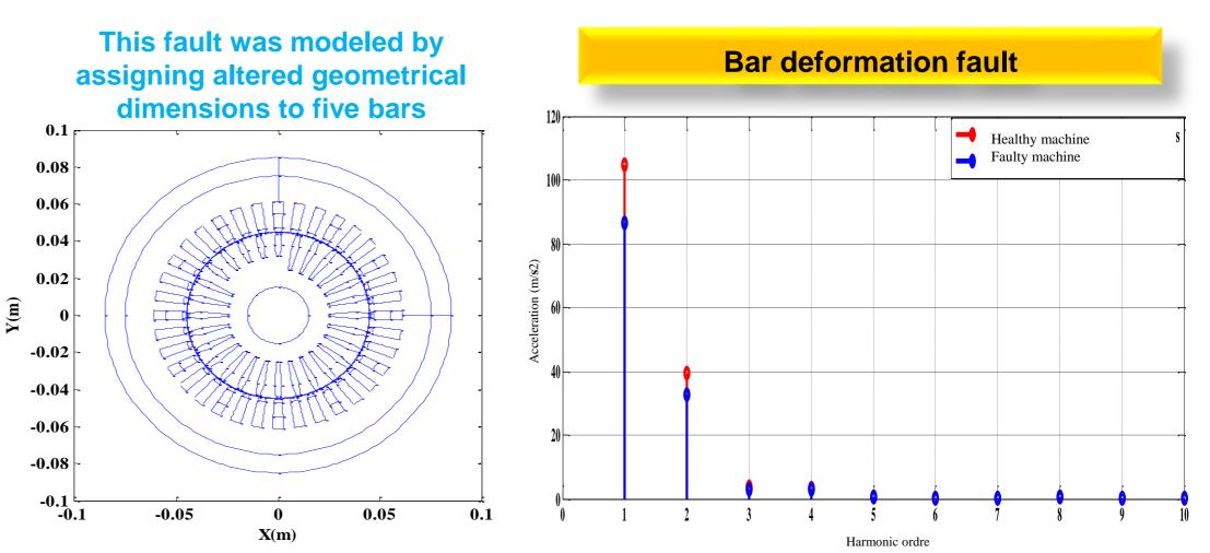
The rise observed in the acceleration spectrum is limited to the fundamental component and the second-order harmonic, with only minor increases in the third- and fourth-order harmonics. These variations result from the non-uniform magnetic field distribution produced by this type of fault.
