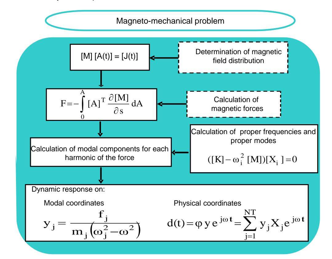
Numerical calculation code based on finite elements method (FEM) was developed under Matlab environment to diagnosing rotor bar breakage, short circuit, bars deformation and other faults. This calculation code was applied in the two cases: when the machine was healthy and when it was faulty.
