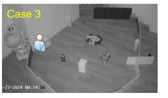
The evaluation show that the mobile platform successfully fulfills its objective, continuously moving and avoiding multiple obstacles without errors or loop failures. Although one collision occurred due to an irregular obstacle, the platform recovered and continued its route. Temperature and motion data clearly indicated when a human target was detected, with readings rising above 30 °C and the motion sensor activating accordingly.
