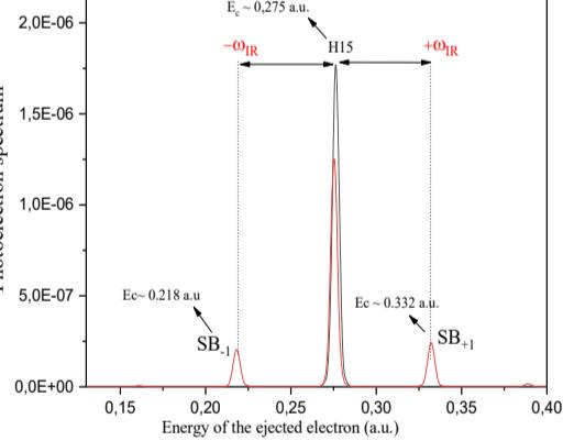
Figure 1: Photoelectron of two-color photoionization of argon ( $m=0$ ). The EUV intensity is  $I_{H15}=10^8 \text{ W/cm}^2$  and the infrared intensity :  $IIR = 0 \text{ W/cm}^2$ ,  $IIR = 5 \times 10^{11} \text{ W/cm}^2$
