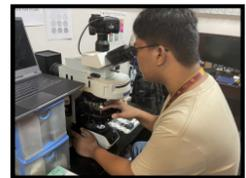
Fig. 3. Point counting using a petrographic microscope
