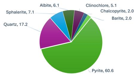
Table 1 - Chemical composition of the material by XRF analysis
