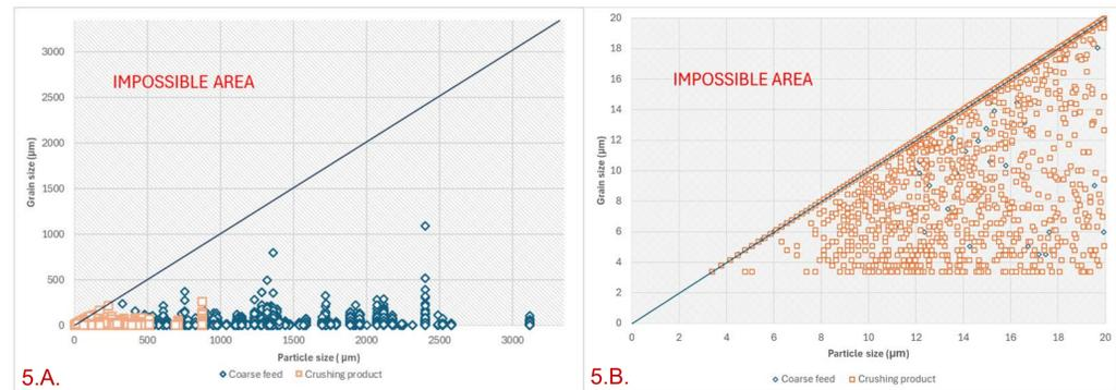
Figure 5 - Grain-particle size relationship for the coarse feed and crushing product indicating the theoretical liberation boundary of chalcopyrite ( $y=x$ ), where: 5.A - View of the entire sample size range (0-3350 μm) and 5.B - Zoomed view of the fine size range (0-20 μm)
