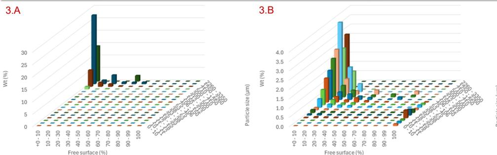
Figure 3 - Distribution of chalcopyrite liberation as mass percentage of particles containing chalcopyrite in the sample, where: 3.A - Free surface in feed and 3.B - Free surface in crushed product
