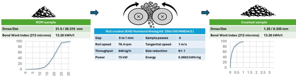
Figure 2 - Operating conditions of the roll crusher and feed-product parameters
