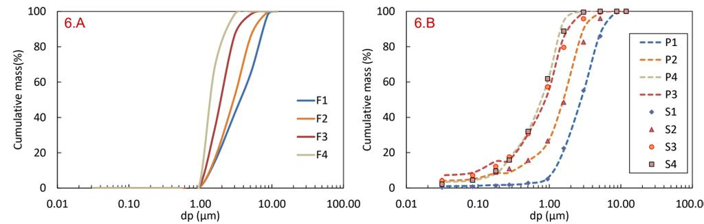
Figure 6 - Breakage modelling of the coarse feed in which: 6.A - PSD of the crusher feed after each stage, where the fine product under 1250 μm of the previous stage has been removed (F1-F4) and 6.B - PSD of the crusher product after each stage (P1-P4) and its simulation through the breakage function (S1-S4)
