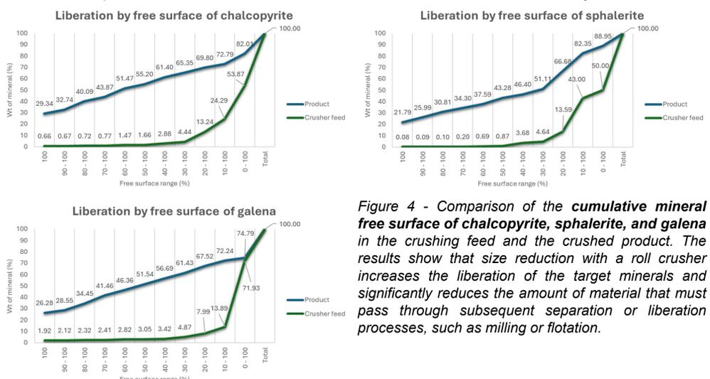
Figure 4 - Comparison of the cumulative mineral free surface of chalcopyrite, sphalerite, and galena in the crushing feed and the crushed product. The results show that size reduction with a roll crusher increases the liberation of the target minerals and significantly reduces the amount of material that must pass through subsequent separation or liberation processes, such as milling or flotation.
