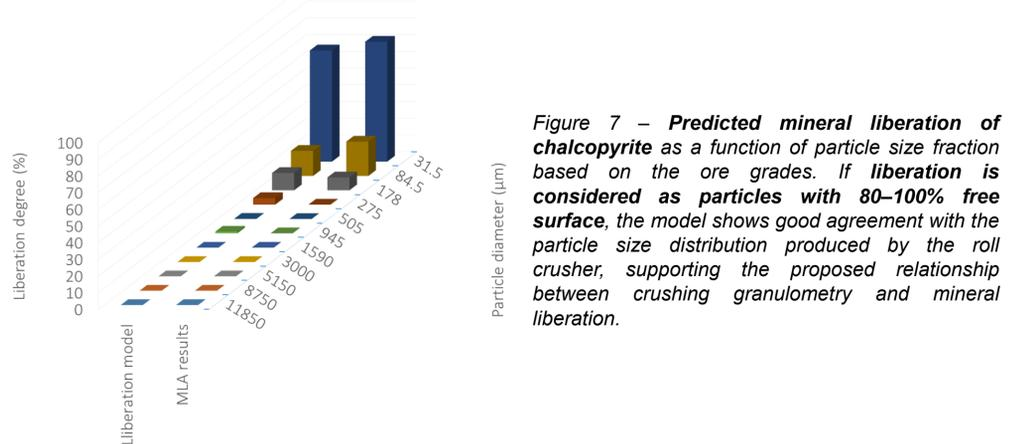
Figure 7 - Predicted mineral liberation of chalcopyrite as a function of particle size fraction based on the ore grades. If liberation is considered as particles with 80-100% free surface, the model shows good agreement with the particle size distribution produced by the roll crusher, supporting the proposed relationship between crushing granulometry and mineral liberation.
