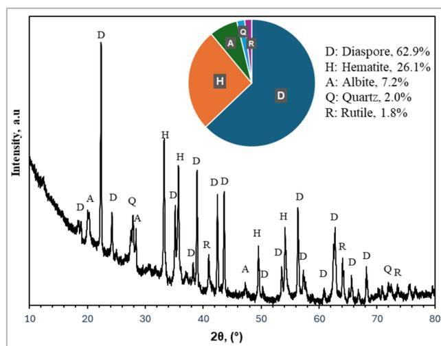
Fig. 1. XRD analysis of Kemiklitepe bauxite ore
