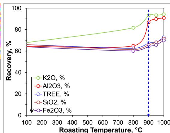
Fig. 4. Recovery of REE and major elements water leaching depending on roasting temperature (75 °C, 15 min, S/O: 15)
