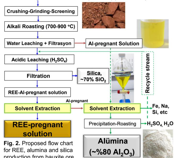
Fig. 2. Proposed flow chart for REE, alumina and silica production from bauxite ore
