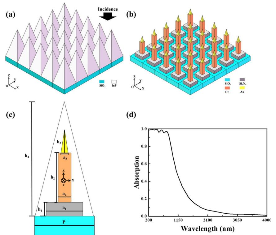
**Figure 1.** (a) External structure of the LWCPA (5×5 array) with incident light along -Z direction; (b) Internal structure of the 5×5 nanocone array; (c) Unit cell cross-section along the X-axis; (d) Theoretical absorption spectrum from 200 nm to 4000 nm.
