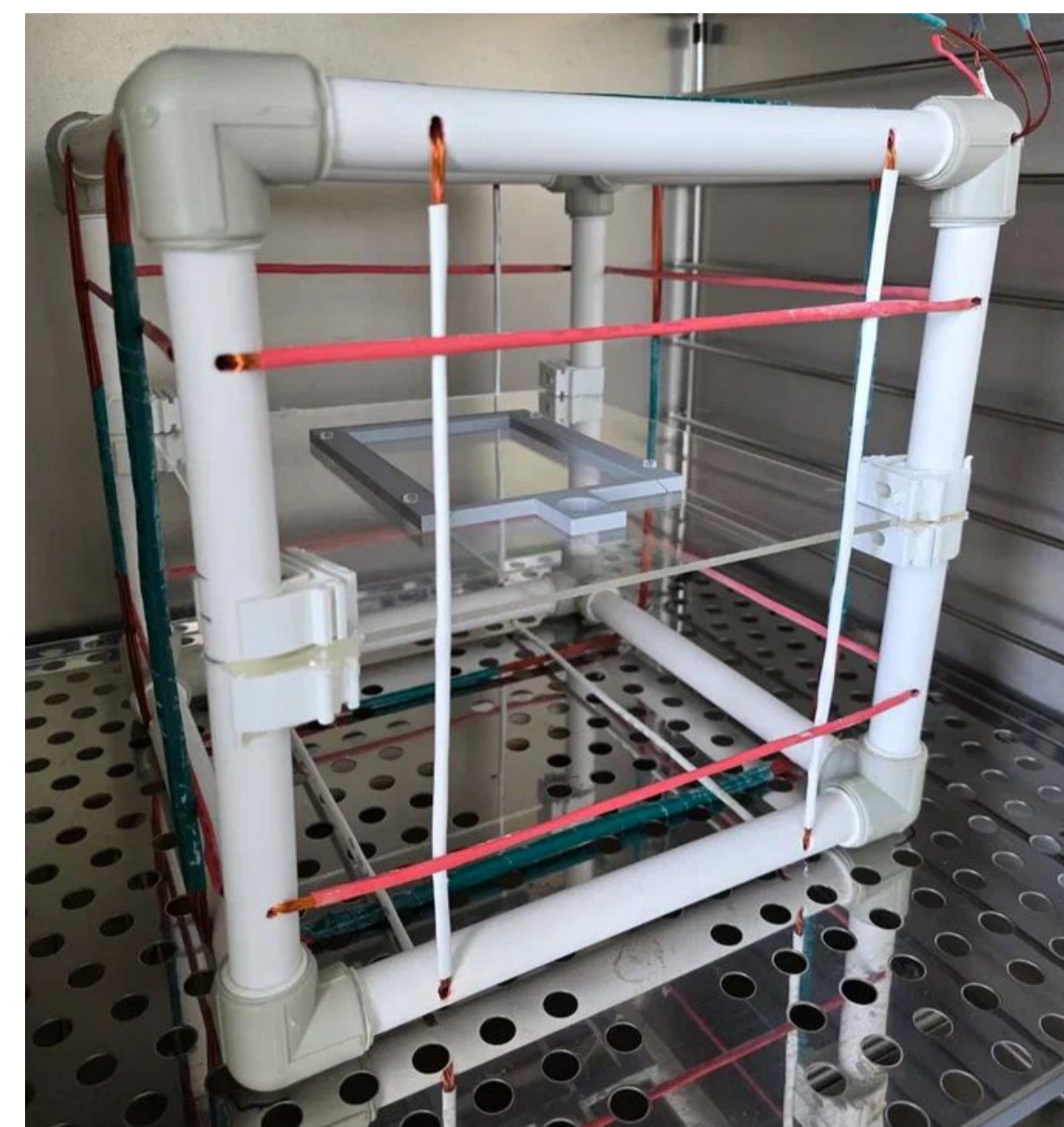
Figure 1. Three-axis Helmholtz coil system with a plate holder in the center, placed inside a BINDER C150 CO 2 incubator.
