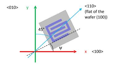
Figure 1. Orientation of membrane and IDTs.
