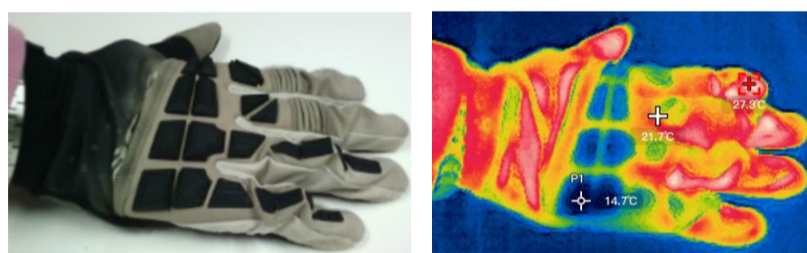
Fig. 2 - Thermal conductivity variation across different regions of a motorcycle glove.
