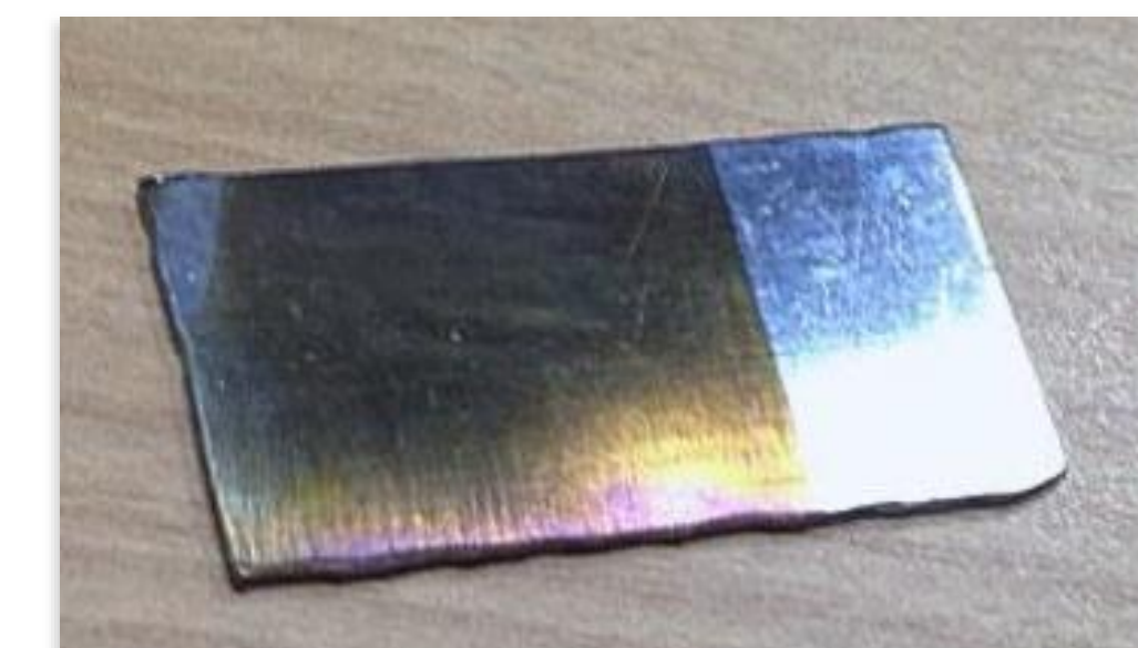
Figure 1: TiO 2 -coated SS316 specimen
