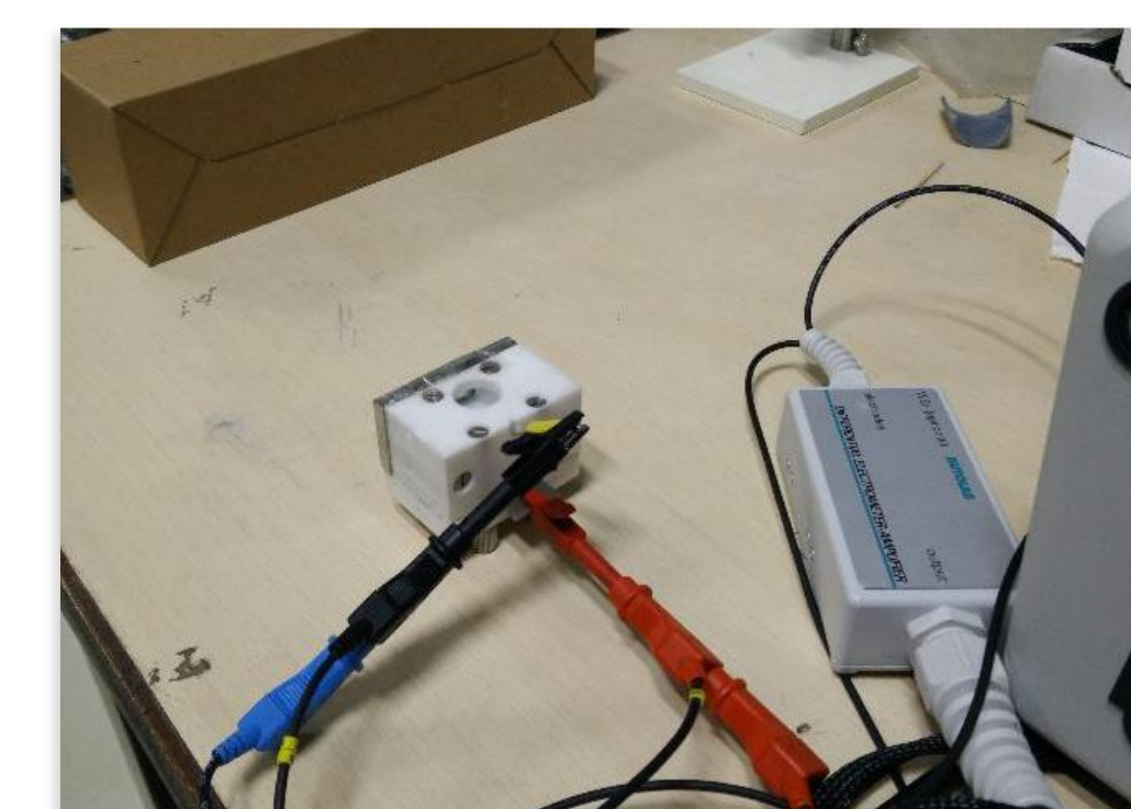
Figure 2: AUTOLAB PGSTAT302N electrochemical cell
