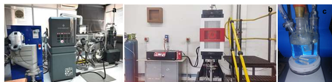
Figure 1: a) shows the photographs of the Amazemate melting machine, b) the Tube furnace and c) the electrochemical test cell.
