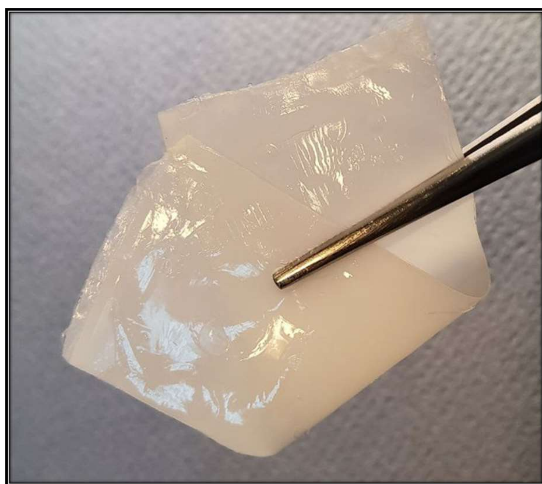
Figure 2. The finished composite bio-patch is a thin, semi-transparent film with a smooth surface, consisting of a PHB matrix coated with an alginate gel.
