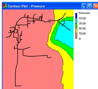
Figure 4. Output in term of pressure for the WDS model without leakages.
