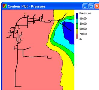
Figure 5. Output in term of pressure for the WDS model with leakage scenario SP1.
