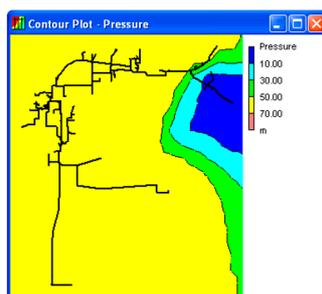
Figure 6. Output in term of pressure for the WDS model with leakage scenario SP8.
