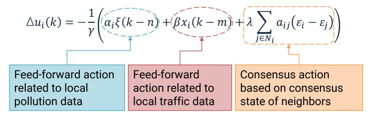
Note: control action is restricted to a variation of  $\pm 50\%$  over the initial value, to avoid large dissimilarities with pre-defined traffic-light cycle lengths.
