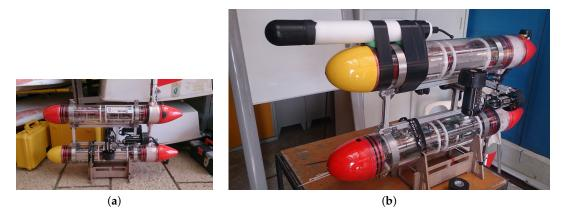
**Figure 3.** (**a**) Photo of the red MEDUSA as operated in this trial and (**b**) turned upside down position with DAVS attached to it.
