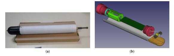
**Figure 1.** (a) Photo of DAVS and (b) exploded view of DAVS in 3D solid modelling, showing the Delrin container (white half tube), the acoustically active part (dark yellow), the two accelerometers (gray blocks), the hydrophone (yellow cylinder), the threaded caps (pink), the electronics (dark green block) and the battery pack (light green).
