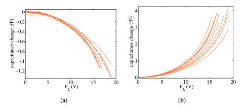
**Figure 3.** Experimental results lateral actuation: (a) LR case (lateral actuation, rotational sensing); (b) LL case (lateral actuation and sensing).
