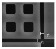
Designed gap Designed beam thickness Beam length  $g_0 = 2 \ \mu m$  $h = 2 \ \mu m$  $l = 20 \ \mu m$
