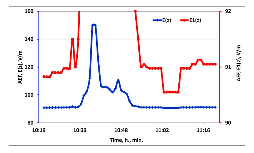
Above the zone of the ore body, a decay of the atmospheric electric field was registered on the order of 100 V/m The reason for the observed decline AEF - hydrogen formed at the top of the ore-body at the expense of electrochemical processes.
