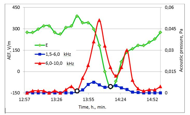
Decay of AEF (increase in radon exhalation) is mainly influenced by acoustic noises of the range 6.0 – 10.0 kHz. Minimal AEF values take place about 30 minutes after the beginning of acoustic noise growth; approximately at the middle of the lifetime of heavy ions. Relatively low AEF values for the railway and its subsequent growth when moving along the profile by ~ 200 V/m are determined by the high level of technogenic seismic noise (5-25 Hz) generated by the movement of the rolling stock.
