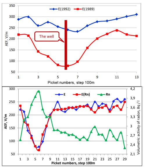
A small subvertical flow of methane is present in plumes of oil deposits. At the 3rd Rechitsa oilfield at the new production well in 1989 and 1992, profile AEF observations were made twice: E (1989) and E (1992)
