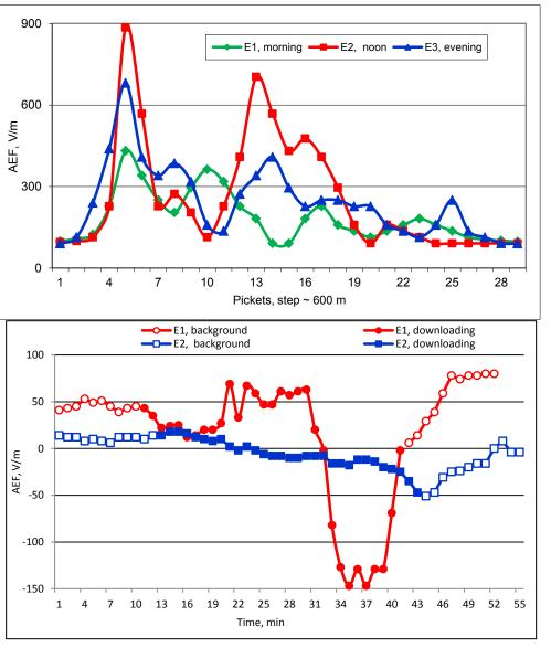
Spatial variations of the AEF on the Svetlogorsk-Uznozh highway over the urban water intake zone. Peak values of the field on the traverse of the intake station ~ 400, 900 and 600 V/m. The reason for this is the depression funnel formed in the reservoir during the water intake
